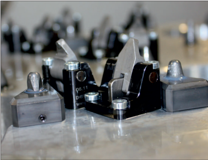
Installation example: multiple workholding fixture with double-acting rotary lever clamps (piston \varnothing 12 mm). For more information and pictures, see page 6.
